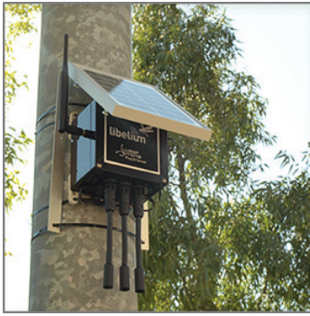
THE SMART SENSOR ABOVE MONITORS AIR QUALITY FOR SMART CITIES.
